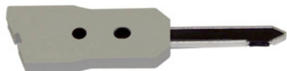
16 or 22 test-plugs, for RTXP 18 or RTXP 24 respectively, which disconnect the relay and connect it to the test leads. Not sold separately.
